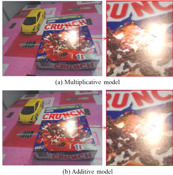
Fig. 8: Comparing the results of our second model CPM using an additive model versus a multiplicative model for computing the illumination variation coefficients.
